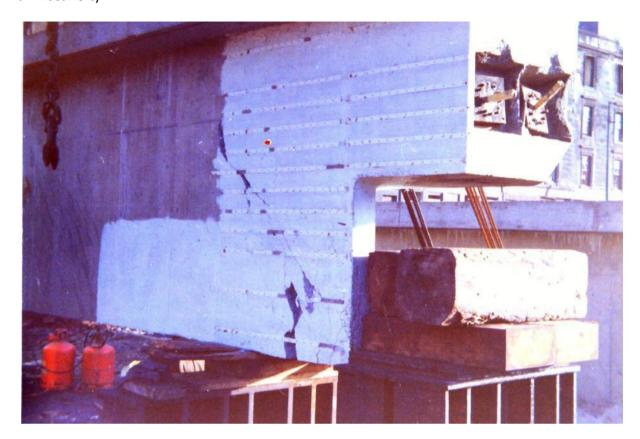
A skewed edge beam half joint on completion of test with jack removed and supported from the underlying ground. Note the steel cable rock anchors, the steel jack support block [resting on the underlying rc pile], the DEMEC strain gauge points and, in this case, the unusual main crack running from the bottom of the beam rather than from the 'root' of the half joint.
